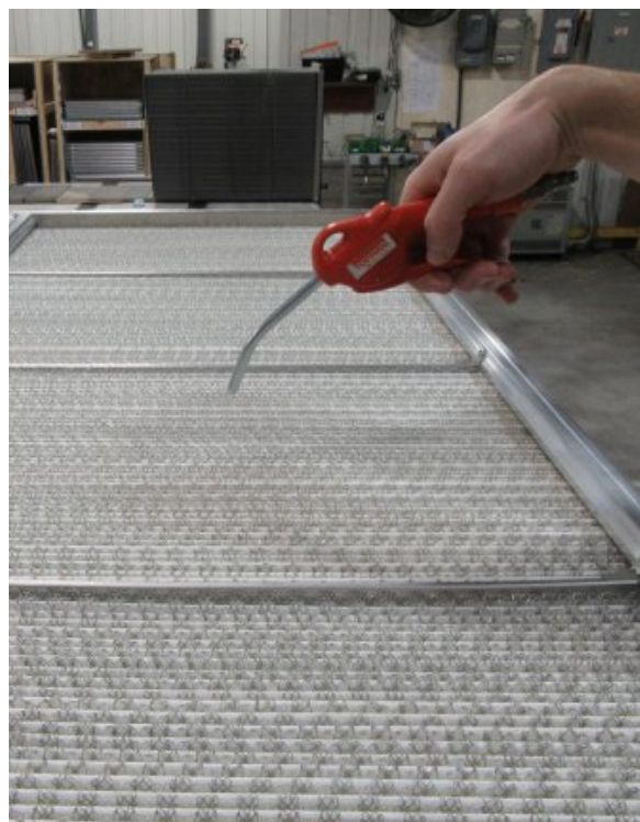
Figure 29 Cleaning with compressed air
