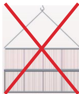
Figure 24 Lifting the IPE5 Exchanger (Incorrect method)
