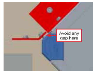
Figure 14 Gaps between the extrusions and the bracket
