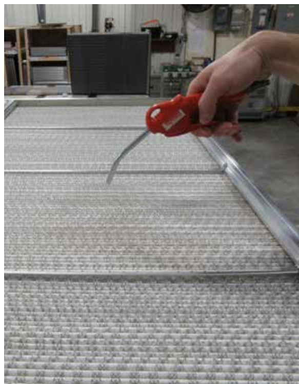
Figure 29 Cleaning with compressed air
