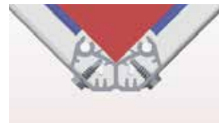
Figure 12 Self-drilling screws through the corner extrusions
