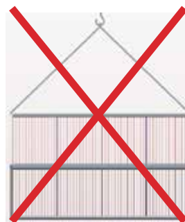
Figure 24 Lifting the IPE5 Exchanger (Incorrect method)
