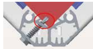
Figure 13 Screws if too long may create leaks!
