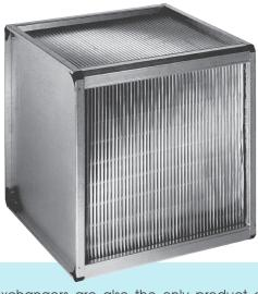
These plate exchangers are also the only product on the market featuring unique mutiple folded plate connections and a special casting sealing method for extremely leakproof assemblies, 100% of the time. Lastly, Hoval plate exchangers highly optimized embossment and folded leading and trailing edges gives them an outstanding rigidity able to resist pressure differentials as high as 10" w.g..
